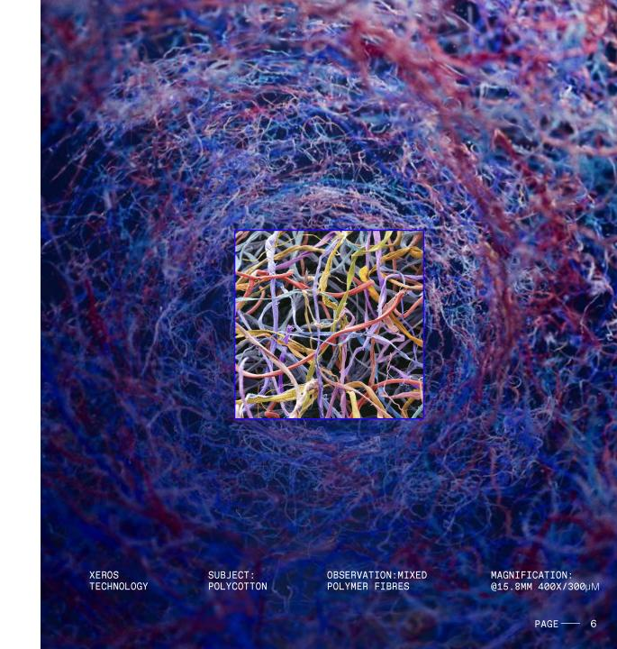
XEROS TECHNOLOGY SUBJECT: MIXED FIBRES OBSERVATION: FINE MESH BARRIER TO MICROPLASTICS
