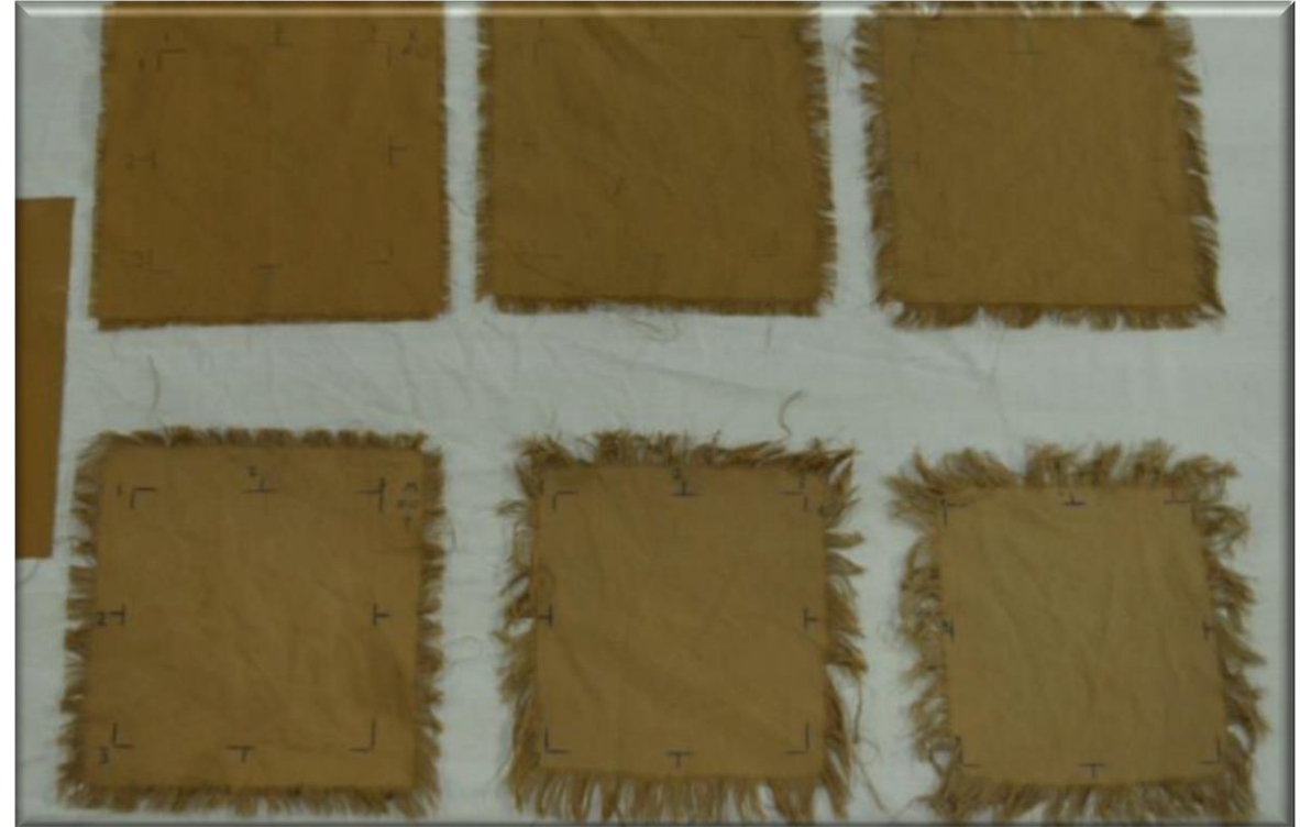
Samples of outer shell firefighter uniform fabric after 10, 30 and 50 washes Xeros process top and conventional process bottom
